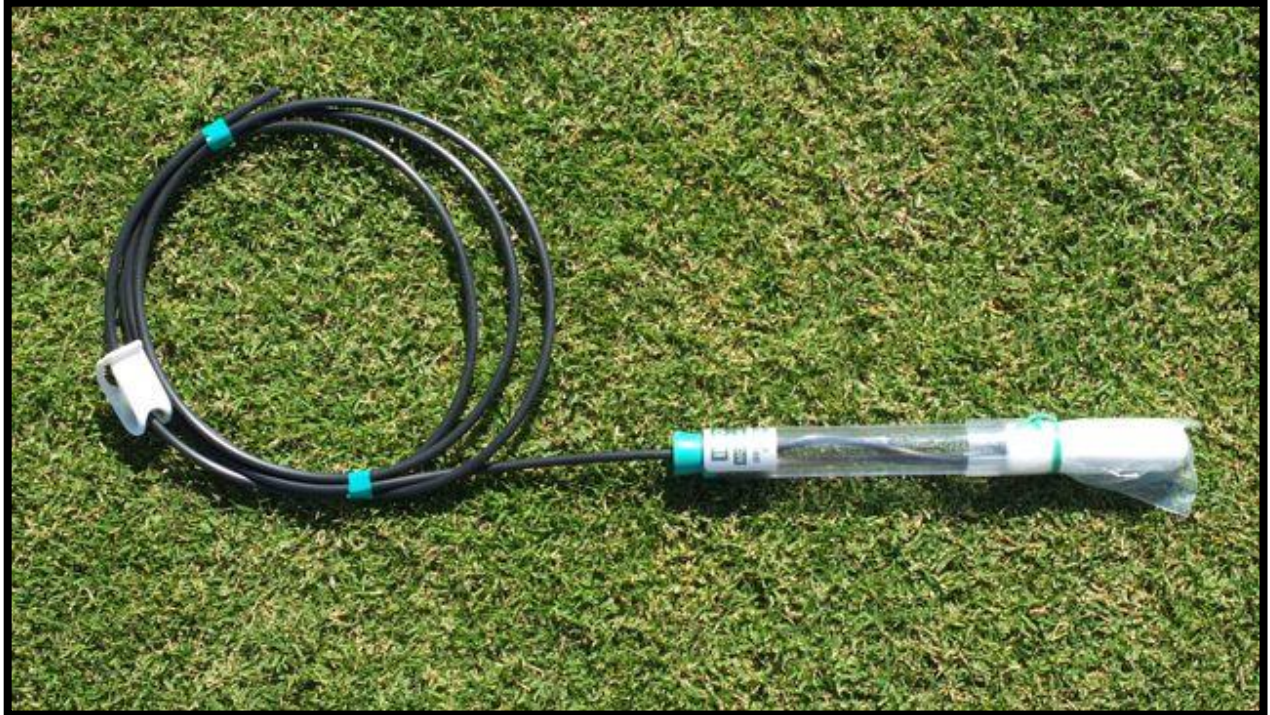
Figure 1. Suction lysimeters (Irrometer, Riverside, CA) used to capture leachate for analysis of EC_L . Lysimeters were buried 4 inches below the turf surface all replicate plots for each treatment in the salinity alleviation study.
