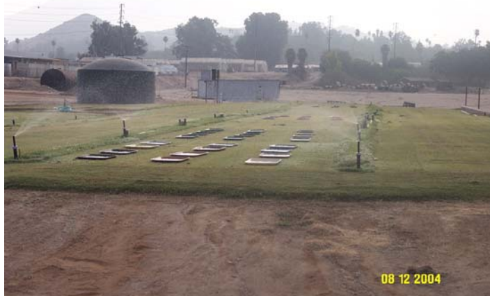
Field study test plots were retrofitted and only recycled water was used for irrigation
