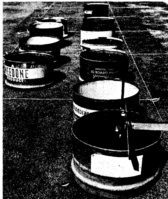
Figure 2. The plot of ring infiltrometers and the book gauge used to record the level of water within the ring infiltrometer.
