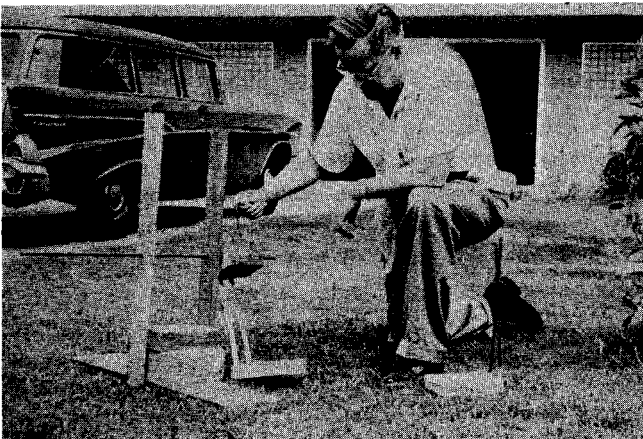
FIG. 1. SIMPLE ONE-PADDLE WEAR-TESTING MACHINE BUILT AS AN EXPERIMENTAL MODEL
